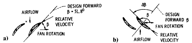
Fig. 3 Fan blade angle convention. a) forward thrust; b) reverse thrust through feather (stall) pitch.
